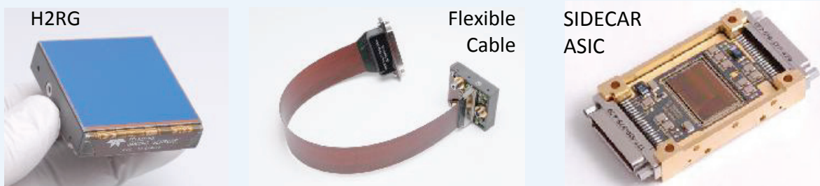
Figure 1: SIDE CAR™ (system image, digitizing, enhancing, controlling, and retrieving) ASIC (Application Specific Integrated Circuit)
