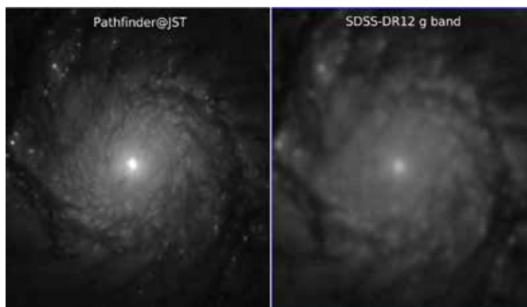
Figure 2: Comparison of the image quality of a coadded image of the central part of M51 resulting from the combination of six 10s single exposures with no filter (left) and the g band image from SDSS (right). The FWHM of the PSF in the Pathfinder image is \sim 0.4'' . The Pathfinder image is a cutout of only 1/30 of the original full frame.
